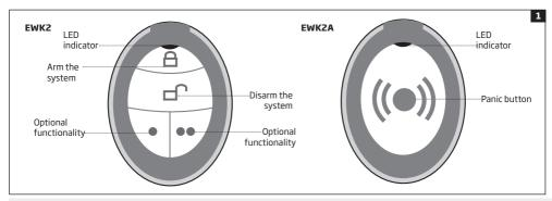
NOTE: Fig. No. 1 reflects the default EWK2/EWK2A button configuration. All EWK2 keyfob buttons are/EWK2A keyfob button is configurable according to individual needs.
